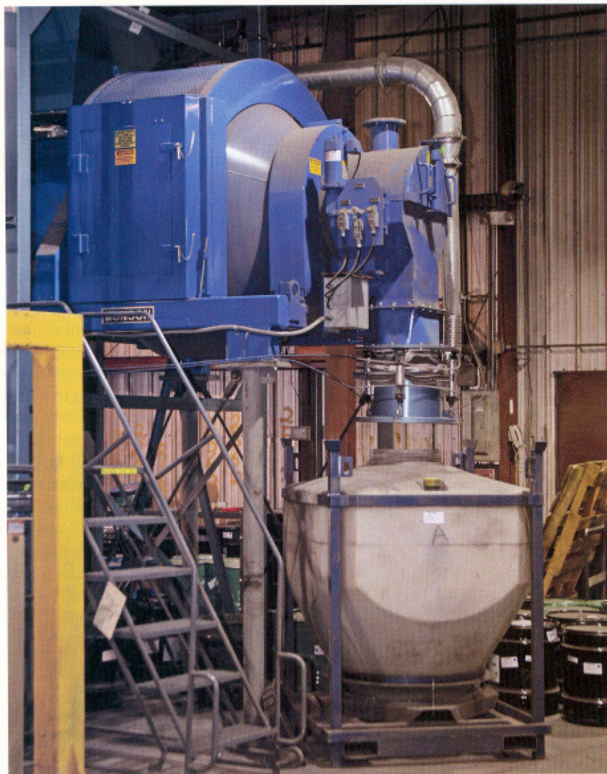
After blending for several minutes, the blender's discharge gate opens and the homogeneously blended metal powders discharge into a bulk drum.
