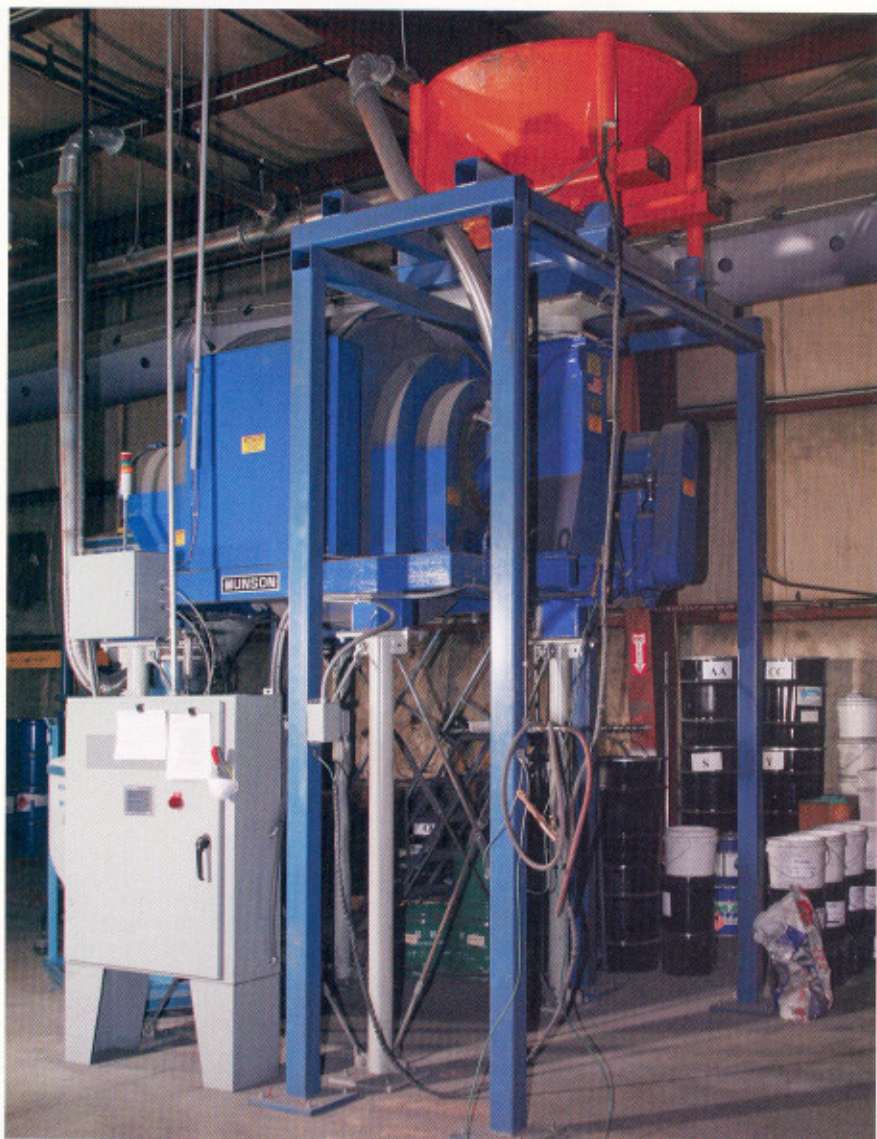
The blender's mixing drum starts rotating before the surge hopper (top, red) discharges the metal powders into it.
